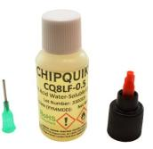
SpecificationsFlux Type:Water Washable Liquid (for Leaded and Lead-Free applications)Flux Classification:ORH1 (Water Soluble, Must be cleaned off post-use using Water or IPA)Specific Gravity:0.85Packaging:15ml Squeeze BottleShelf Life:Refrigerated >24 months, Unrefrigerated >24 months
