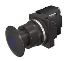
30mm BlackMax, Epoxy Coated Corrosion Resistant Complete Metal Unit Illuminated Push-Pull Operator Full Voltage, 24V AC/DC Incandescent Lamp Mushroom Head Cap Small 1 3/4" (44.5 mm) Metal, Black with Blue Lens 3 Position Pull-Momentary/Push-Maintained UL Listed, CSA Certified NEMA 1,3,3R,4,4X,12,13 & Automotive Standards
