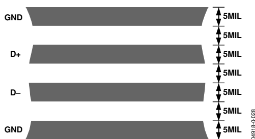
Figure 29. Arrangement of Signal Tracks
