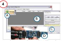
Launch Sense and Control Dashboard and 'bind' the RF Expansion board.
