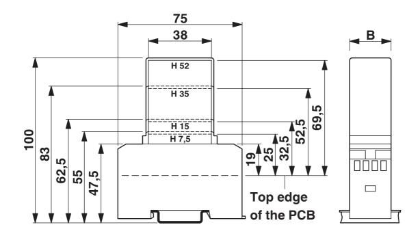
1 = Top edge of the PCB B = Housing width
