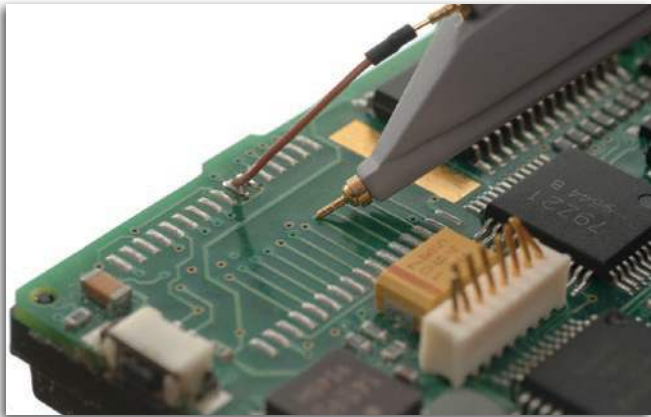
Use the Solder-In Ground with Straight Tip for general purpose browsing.
