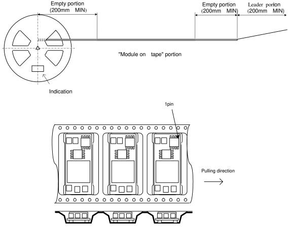
The module is located such as parts in upper side and substrate in lower side.
