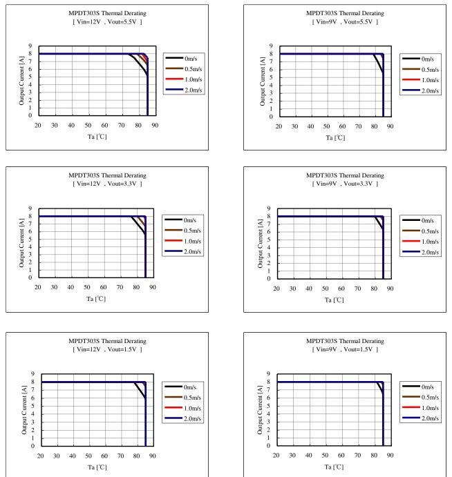
The above derating limits apply to this product soldered directly to 101.6×180mm×1.6mm PCB (double-sided, with 70um copper). Any adjacent parts of high temperature or difference of PCB design may cause overheat of this product. For reliable operation, please check that the FETs temperature of this product is below 120 °C, and the inductor temperature of this product is below 110 °C.
