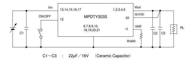
**Ripple Noise Measurement Circuit**
