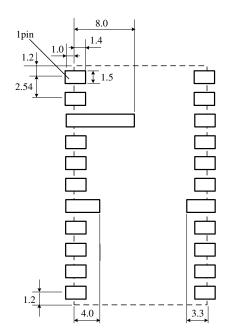
There are wiring coppers or through-hole via at the bottom side of the DC-DC Converter. When you design your PCBs, please be careful not to short the circuit of the DC-DC Converter or PCBs.
