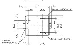
\* The terminal position or intervals between terminals is measured at A surface level.
