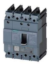
circuit breaker 3VA5 UL frame 125 breaking capacity class S 25kA @ 480V 4-pole, line protection TM230, FTAM, In=110A overload protection Ir=110A fixed short-circuit protection Ii=5...10 x In N conductor protection 100% without connection
