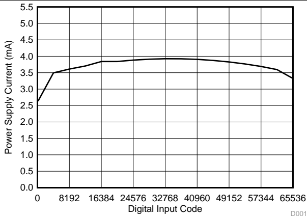
Figure 33. Power Supply Current vs Digital Input Code
