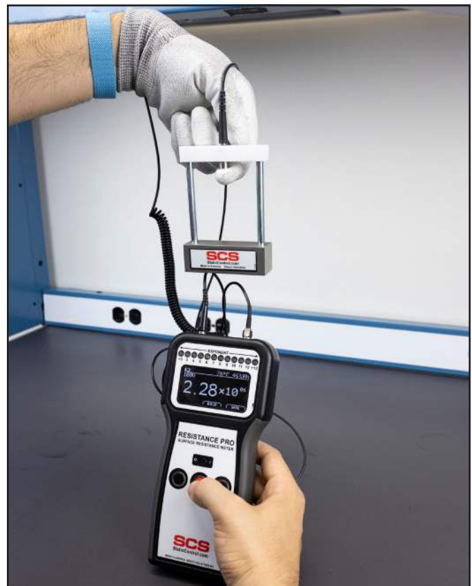
Figure 2. Using the Glove CAFE Test Electrode with the SCS 770760 Resistance Pro Meter
