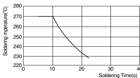
[Allowable Flow Soldering Temperature and Time]
