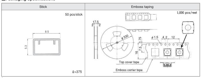
When ordering, tape packaged version shall be supplied by request. Minimum packaging quantity for reel packaging is 1,000pcs per reel.
