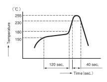
· Apply reflow soldering up to 2 times max.
