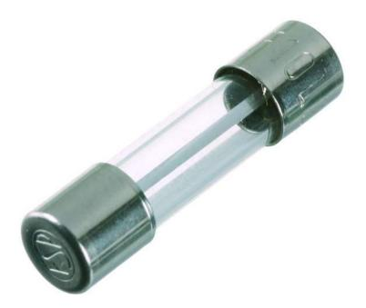
Fuse, Dimensions: 5x20 mm, Trigger characteristic: Slow-acting (T); Rated voltage: 250 V, Rated current: 6.3 A
