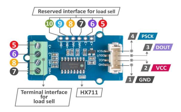
1 : Connected to the system GND
