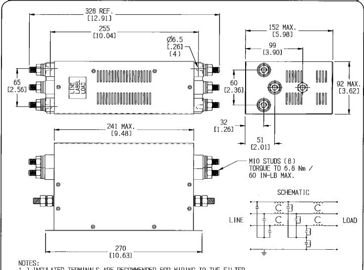
1.) INSULATED TERMINALS ARE RECOMMENDED FOR WIRING TO THE FILTER
