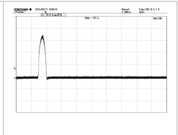
Figure 8: Inrush current @ Vin=220Vac lin: 10A/div, 5mS/div
