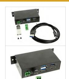
USB C hub provides 4 USB 3.1 Gen1 ports to include 3 USB-A ports and 1 USB C port. 1 Downstream and 1 upstream port use the reversible USB C connector. USB C hub is a Gen1 hub using USB 3.1 to support Super-Speed 5Gbps data transmission speeds and takes advantage of the reversible type-C port in both directions. This hub is self powered with a 2-pin terminal block connector to supply power input of  $+7 \sim 48V$  DC sold separately.
