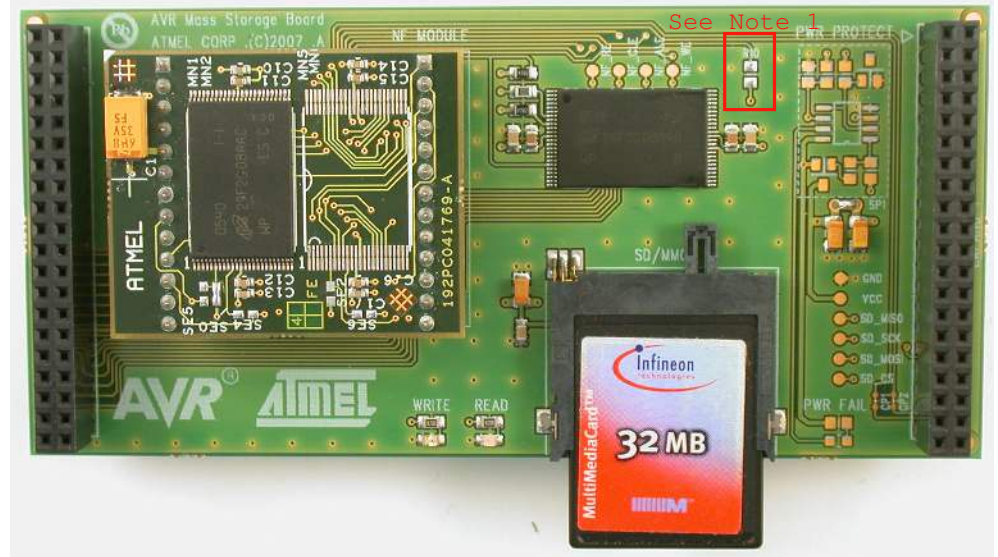
NF Module Installation Figure 2-5 . NAND Flash module on the ATEVK525, plus MMC card
