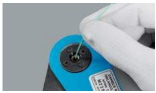
Insert the wire into the contact.
