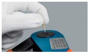
Insert the contact into the crimping tool.
