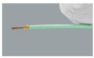
Strip the insulation from the copper wire, with 5 mm maximum strip length. (For aluminum wire, consult TE.)
