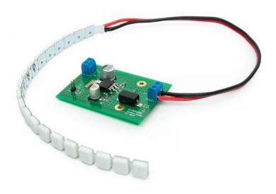
Dione Maxi consists of an array of MEMS speakers and the external amplifier to drive them. The speaker array, which is also referred to as the sound stripe, includes 20 USound Adap speakers connected in parallel. Due to its flexible structure and protective construction, the sound stripe is ideal for applications where audio is added on top of an existing design.
