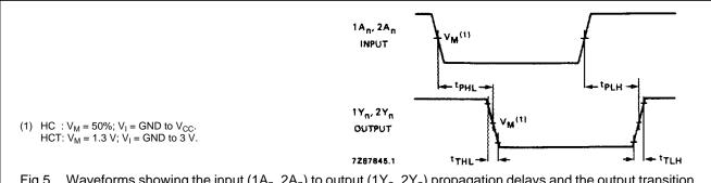
Fig.5 Waveforms showing the input (1A<sub>n</sub>, 2A<sub>n</sub>) to output (1Y<sub>n</sub>, 2Y<sub>n</sub>) propagation delays and the output transition times.
