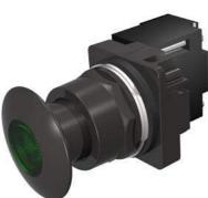
30mm BlackMax, Epoxy Coated Corrosion Resistant Complete Metal Unit Illuminated Push-Pull Operator Transformer type, 600V AC Incandescent Lamp Mushroom Head Cap Small 1 3/4" (44.5 mm) Metal, Black with Green Lens 2 Position Maintained, Pull-to-Release UL Listed, CSA Certified NEMA 1,3,3R,4,4X,12,13 & Automotive Standards
