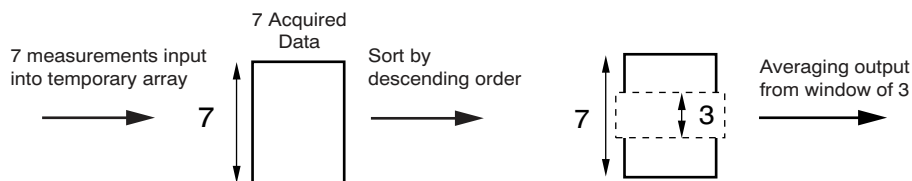
Figure 28. MAV Filter Operation (Patent Pending)
