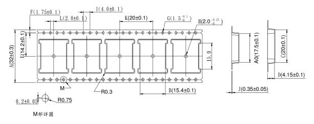
Note: Tolerances unless mentioned ±0.25mm. Unit = mm
