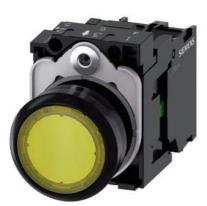
Illuminated pushbutton, 22 mm, round, plastic, yellow, pushbutton, flat, momentary contact type, with holder, 1 NO, LED module with integrated LED 230 V AC, screw terminal
