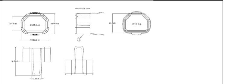
Warning: When removing connector with this sleeve included, take care not to damage the inlet when removing the connector. To remove the Sleeve that remains in the inlet after cord extraction, ensure the power cord is not plugged into power and use a non-conductive tool to extract.
