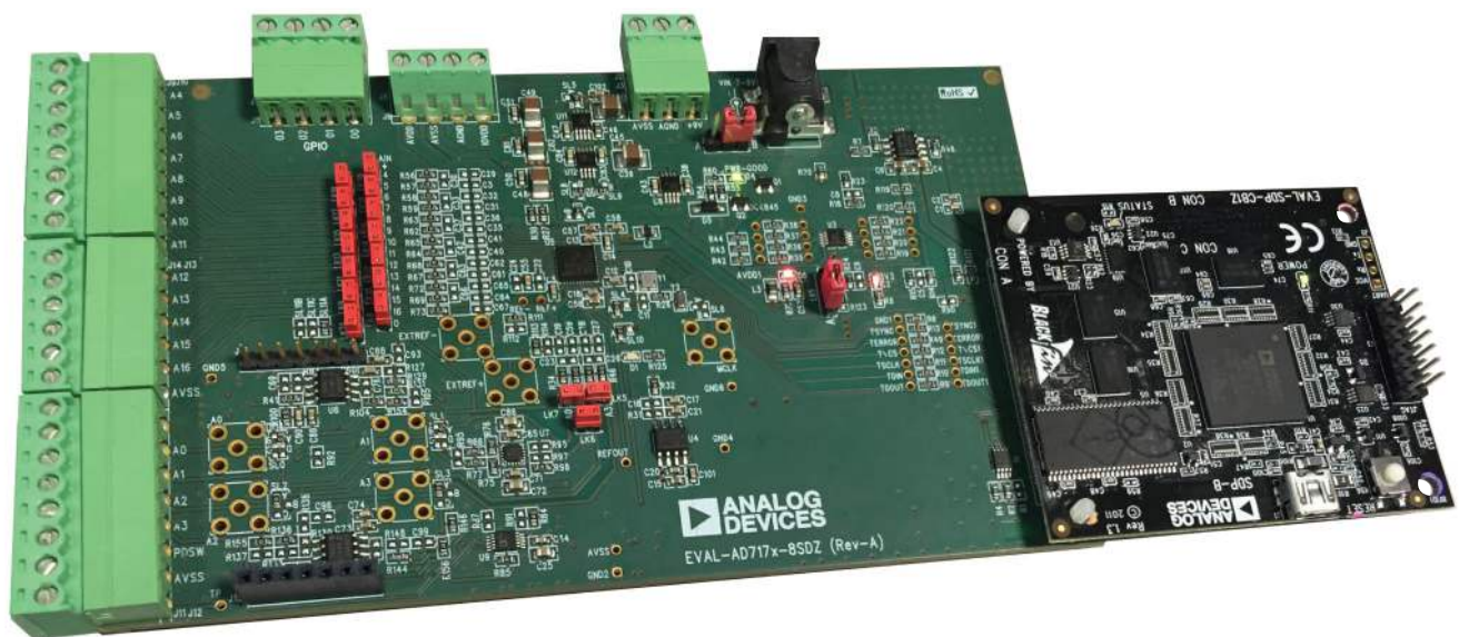
Figure 2. Hardware Configuration, Setting Up the EVAL-AD7175-8SDZ
