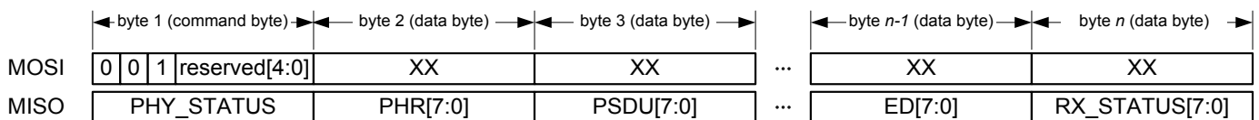
Figure 6-7. Packet Structure - Frame Read Access.
