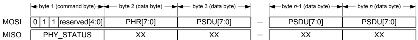
Figure 6-8. Packet Structure - Frame Write Access.
