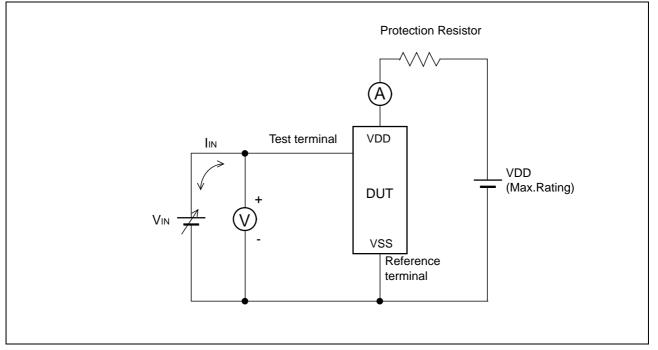
Note : The voltage VIN is increased gradually and the current IIN of 300 mA at maximum shall flow. Confirm the latch up does not occur under  $I_{IN} = \pm 300$  mA. In case the specific requirement is specified for I/O and IIN cannot be 300 mA, the voltage shall be
