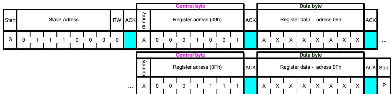
Figure 15: I 2 C multiple write protocol
