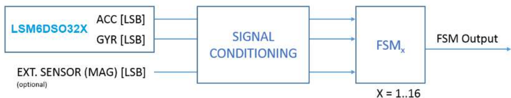
Figure 2. State machine in the LSM6DSO32X
