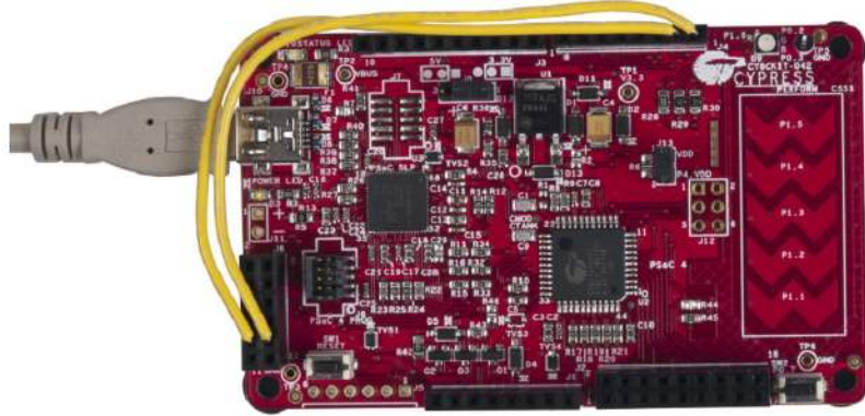
Figure 6-10. UART Connection Between PSoC 4 and PSoC 5LP
