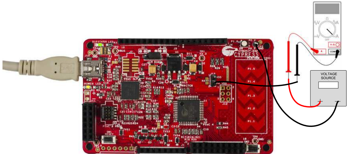
Figure 4-6. PSoC 4 Current Measurement when Powered Separately
