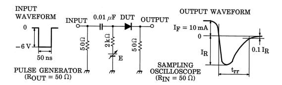
Fig.1 Reverse Recovery Time (t<sub>rr</sub>) Test Circuit
