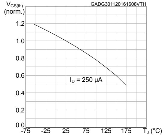
Figure 8. Normalized gate threshold voltage vs temperature
