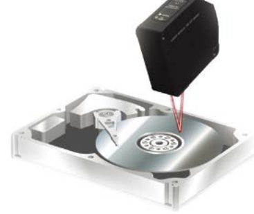
Measurement of HDD surface variations
