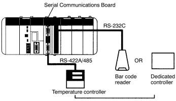
Standard external devices with an RS-232C or RS-422A/485 port
