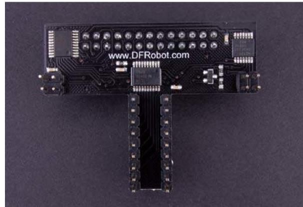
Note: For medium-size breadboards, the interface is not aligned with the middle of the bread, please insert the left power pins on top left while needle skip down one hole with the right power pin, as shown in picture.
