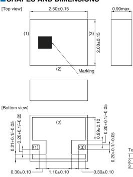
Terminal functions Input / Output Port Output / Input Port
