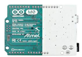
The Arduino M0 is ideal for projects demanding high computing power. It features a Cortex M0+ running at 48MHz clock speed. All digital pins have PWM capability. It also has a real digital to analog conversion making it ideal for sound applications
