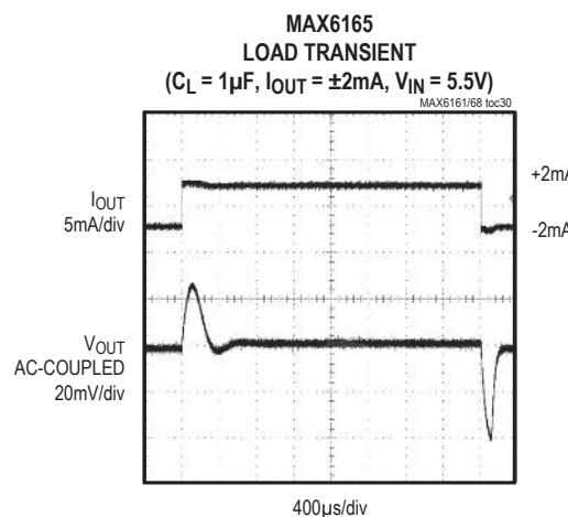
**Typical Operating Characteristics (continued)**(V<sub>IN</sub> = +5V for MAX6161–MAX6168, V<sub>IN</sub> = +5.5V for MAX6165, I<sub>OUT</sub> = 0, T<sub>A</sub> = +25°C, unless otherwise noted.) (Note 5)
