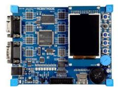
The Keil MCBSTM32EXL Evaluation Boards enable you to create and test working programs based on the STMicroelectronics STM32 family of ARM Cortex<sup>™</sup>-M3 processor-based devices.
