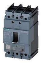
circuit breaker 3VA5 UL frame 125 breaking capacity class S 25kA @ 480 V 3-pole, line protection TM230, FTAM, In=25A overload protection Ir=25A fixed short-circuit protection Ii=6...12 x In UL489 SB (naval), 50 deg. cel. nut keeper kit on both sides
