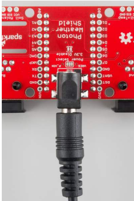
Powered through the Barrel Jack.
