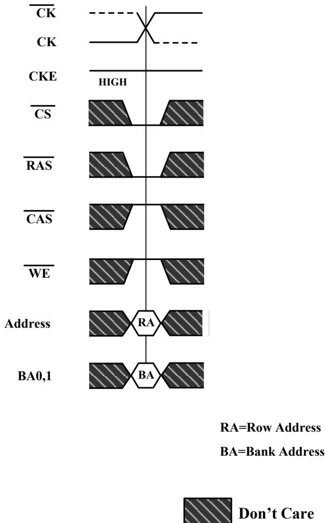
**Figure 5. t<sub>RCD</sub> and t<sub>RRD</sub> Definition**
