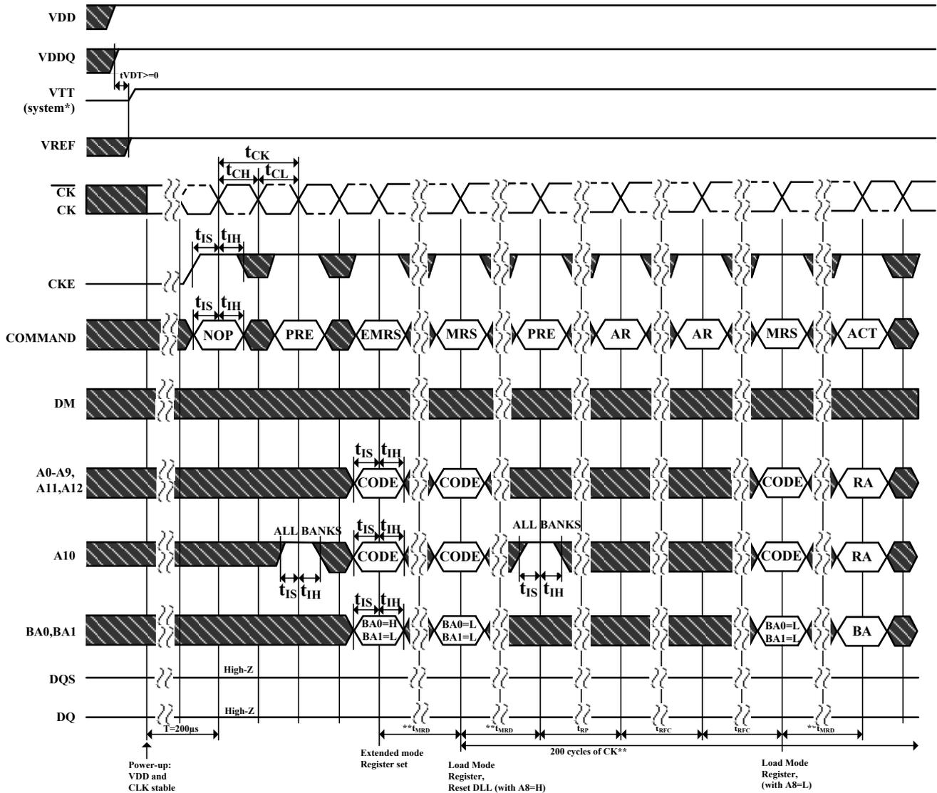
\*=VTT is not applied directly to the device, however  $t_{VTD}$  must be greater than or equal to zero to avoid device latch-up
