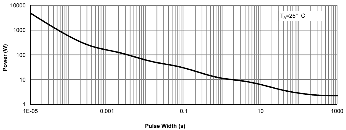
Figure 14: Single Pulse Power Rating Junction-to-Ambient (Note H)
