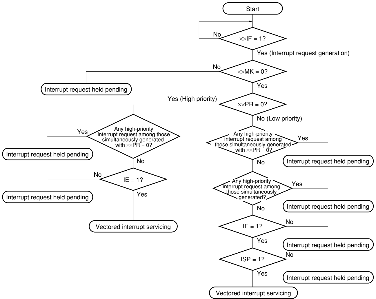
Figure 19-10. Interrupt Request Acknowledgment Processing Algorithm
