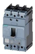
circuit breaker 3VA5 UL frame 125 breaking capacity class S 25kA @ 480 V 3-pole, line protection TM230, FTAM, In=30A overload protection Ir=30A fixed short-circuit protection Ii=5...10 x In UL489 SB (naval), 50 deg. cel. cable connection on both sides
