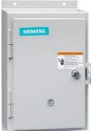
Non-reversing motor starter, Size 0, Three phase full voltage, Solid-state overload relay, OLRelay amp range 5.5-22a, 110V 50HZ / 120V 60HZ coil, Non-combination type, Enclosure type 12, Dust/drip proof for indoors, Extra-wide enclosure
