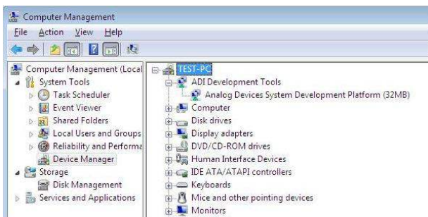
Figure 13. Device Manager: Checking that the Board Is Connected to the PC Correctly
